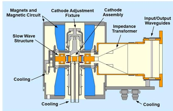
**Cross section of a CFA**
