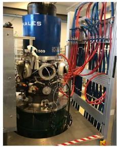
1 MW, 170 GHz gyrotron
